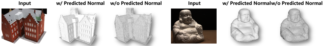
Figure 7: WorldMirror Improves Surface Reconstruction with Predicted Normal Maps.
