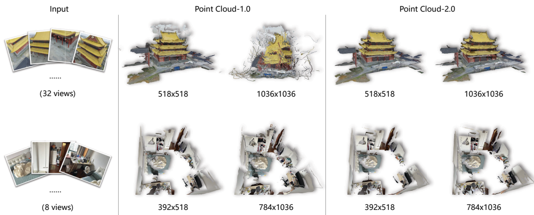
Figure 26: Multi-resolution point cloud comparison of WorldMirror 1.0 and 2.0. We evaluate under dense (32 views, top) and sparse (8 views, bottom) settings at different inference resolutions. WorldMirror 1.0 degrades severely at high resolution, while WorldMirror 2.0 maintains consistent reconstruction quality across all resolutions.
